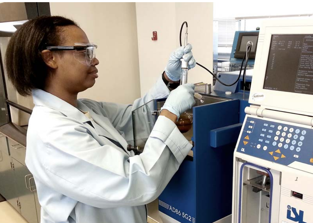
Army Sgt. Deliscia St. Clair, a petroleum laboratory technician at the DLA Energy Alaska lab in Anchorage, tests a sample of jet fuel on a distillation machine. The lab tests mainly jet fuels, like JP-4 and JP-5, which are cold-weather fuels that contain additives to help aircraft deal with the extreme cold in northern Alaska.
